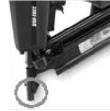
Don't tamper with safety features
